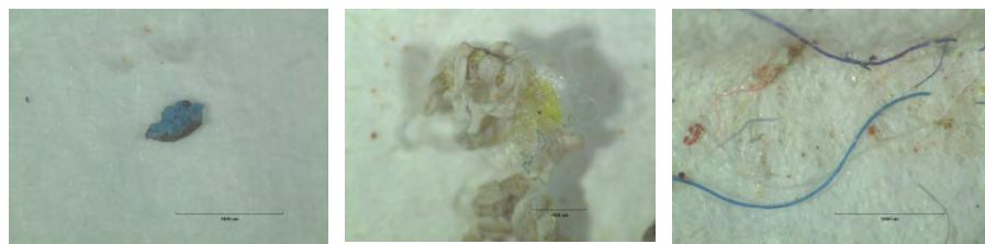
Figure 3. Example of microplastic pictures: fragments (left and centre), fibres (right).
