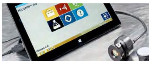
Figure 4. MicroNIR Pro 1700. Wavelength range 950 – 1650 nm; size 4.5x5 cm, 64 g.
